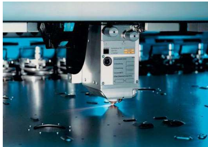
Precise contours achieved by a combination of stamping and laser cutting
