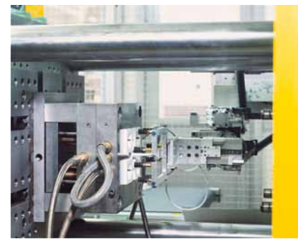
Production at Gira: the company is one of the first worldwide to use ARBURG’s combined technology with the ALLROUNDER injection moulding technology and the MULTILIFT H handling system.
