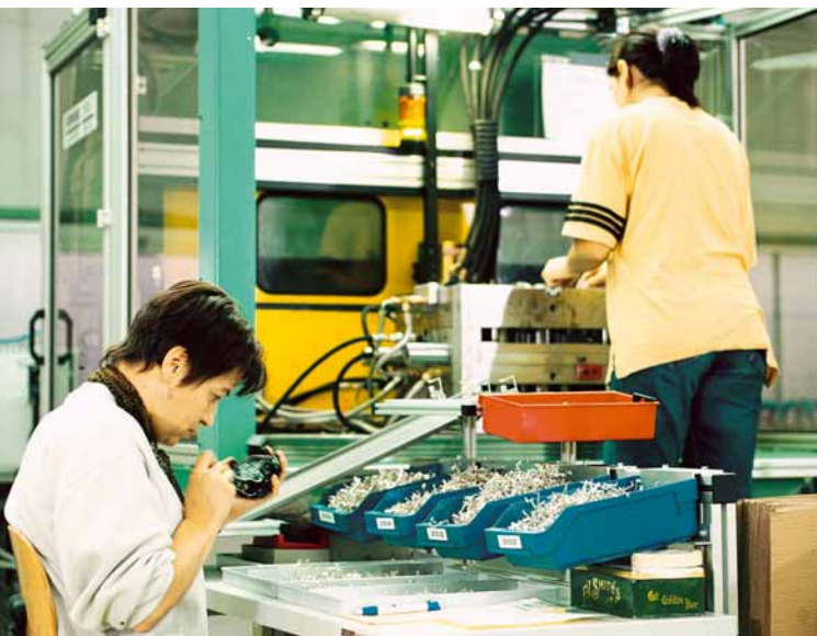
Inserting the metal inserts into the mould station on the rotary table machine (r.) and the visual inspection of moulded parts afterwards.
