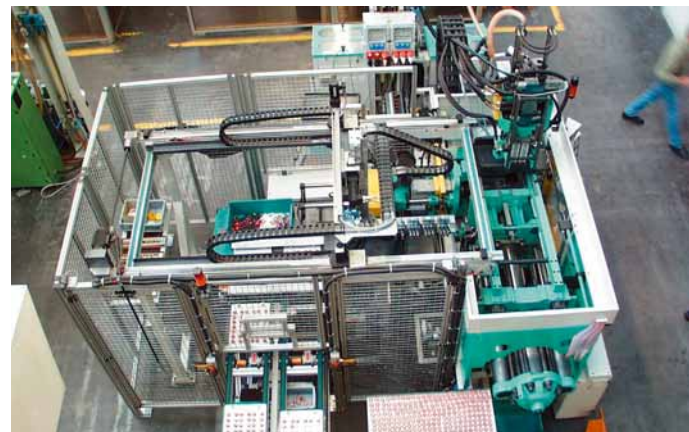
The right tool for the job: an ALLROUNDER 420 C for three-component processing: integrated into a production cell for manufacturing pistons for cylinders.
