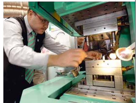
Insertion of the inserts and removal of the finished moulded parts can also be performed manually with the ALLROUNDER V.
