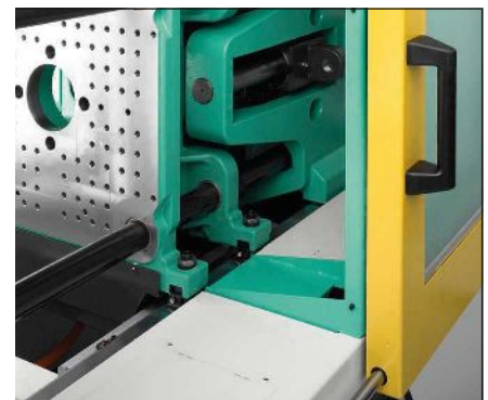
Above: The safety guard is enlarged at the rear to offer more space.
